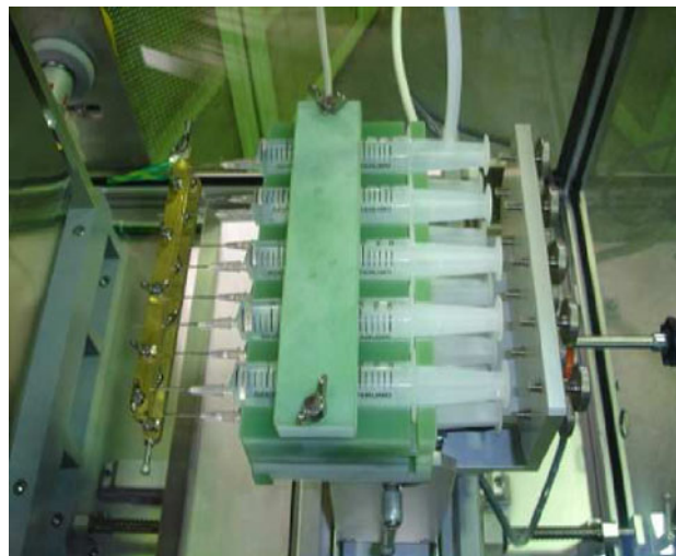
Fig. 1 Apparatus of multi-jet electro-spinning with a group of syringes and nozzles
